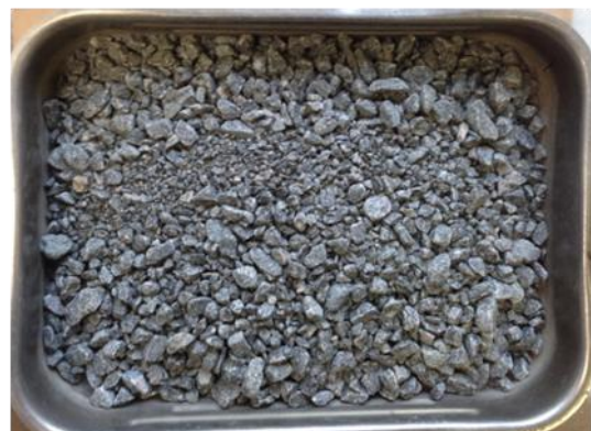
Figure D.2 145308 Crushed rock base course gneiss 1 Angered
