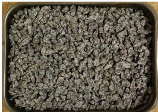
Figure D.14 145280 Crushed rock cobbles Bohus Granite Tanum
