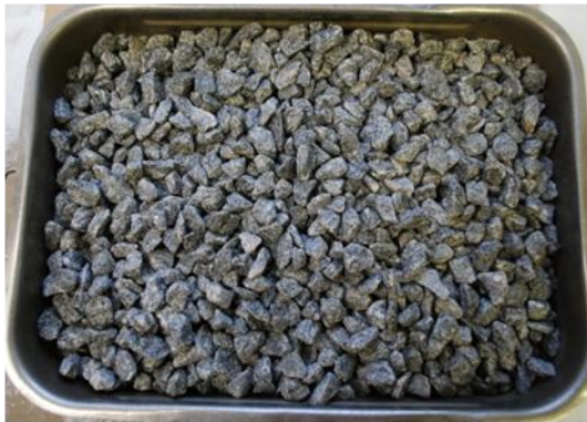
Figure D.2 145308 Crushed rock base course gneiss 1 Angered
