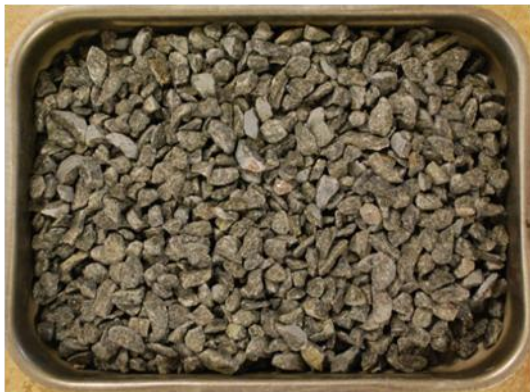
Figure D.3 145283 Rock core gneiss 2 Angered
