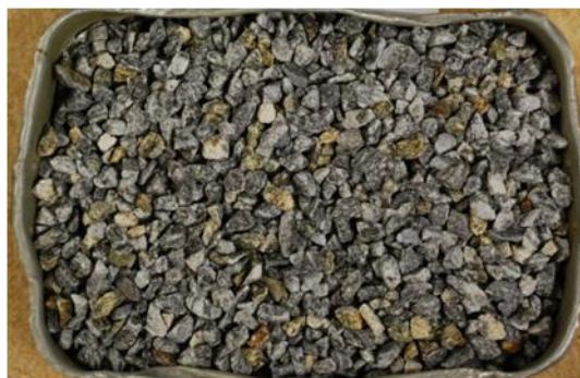
Figure D.11 145263 Rock core gneiss Tanum
