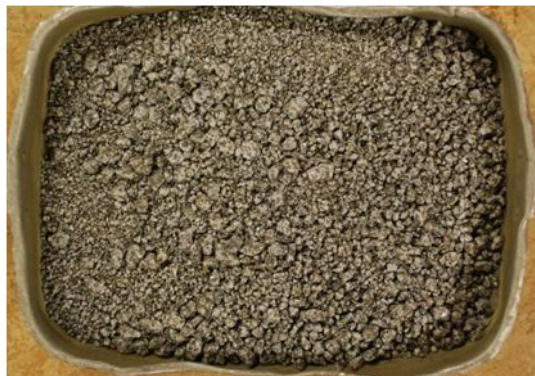
Figure D.14 145280 Crushed rock cobbles Bohus Granite Tanum
