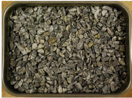
Figure D.12 145279 Crushed rock cobbles gneiss Tanum
