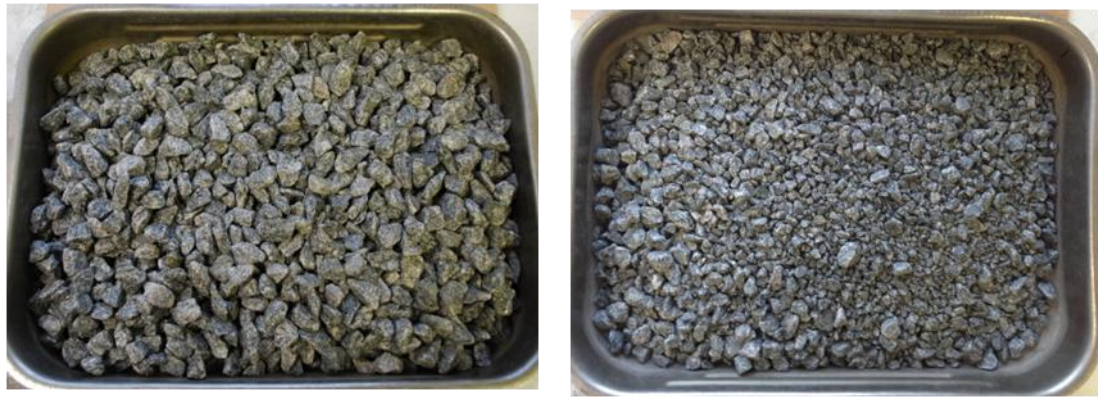
Figure D.4 145309 Crushed rock base course gneiss 2 Angered
