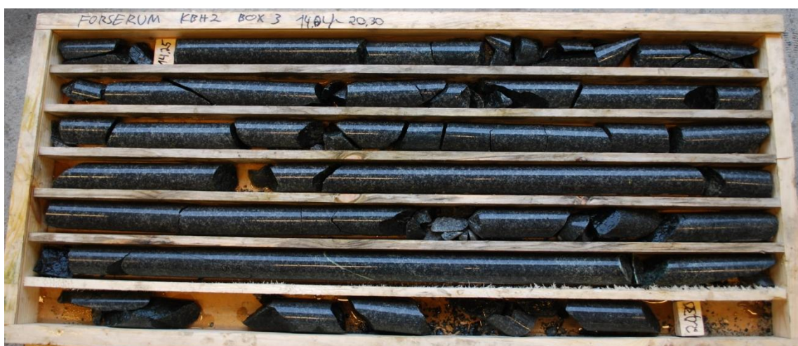
Figure B.35 Forserum KBH2 Box 3 [14.04–20.30 m]
