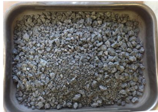
Figure D.2 145308 Crushed rock base course gneiss 1 Angered
