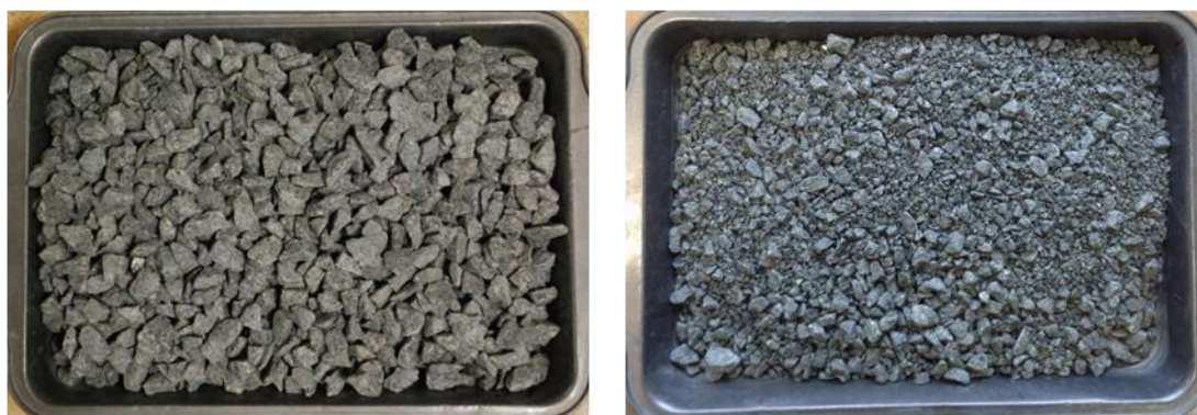
Figure D.20 145265 Crushed rock base course dolerite 2 Forserum
